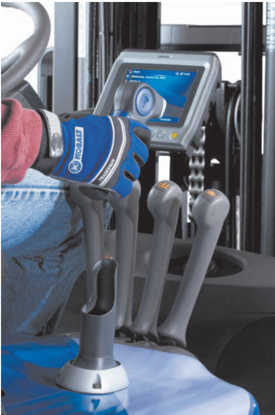
FIGURE 2-8 In an efficient warehouse, smart forklifts can read RFID tags or UPC numbers and transmit data to a CRM system.
