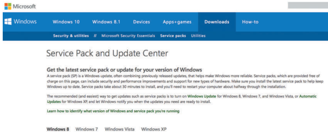
FIGURE 12-12 A Microsoft service pack provides access to updated drivers, tools, security patches, and customer-requested product changes.
