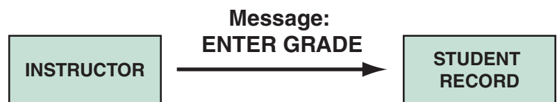
FIGURE 6-6 In a school information system, an INSTRUCTOR object sends an ENTER GRADE message to an instance of the STUDENT RECORD class.
