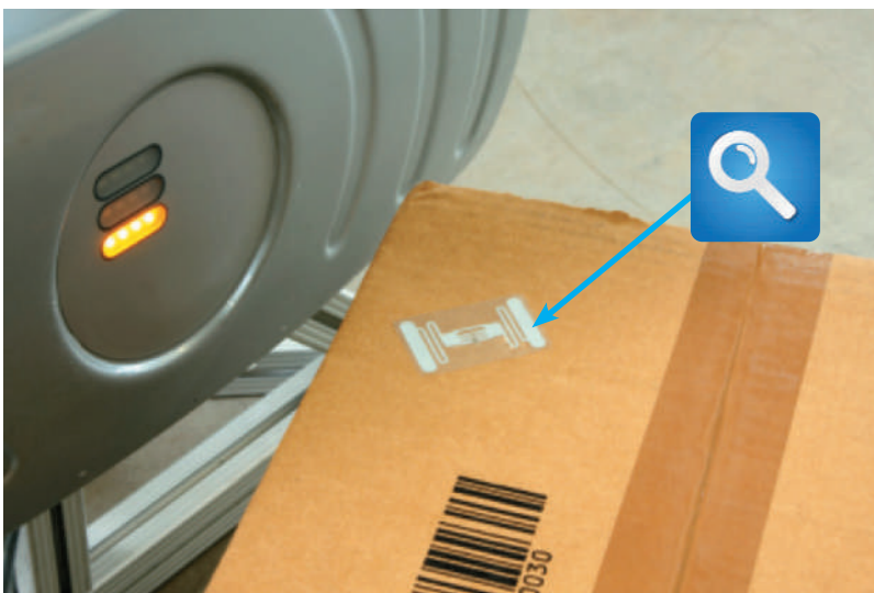
FIGURE 1-12 With an RFID tag, items can be tracked and monitored throughout the shipping process.
